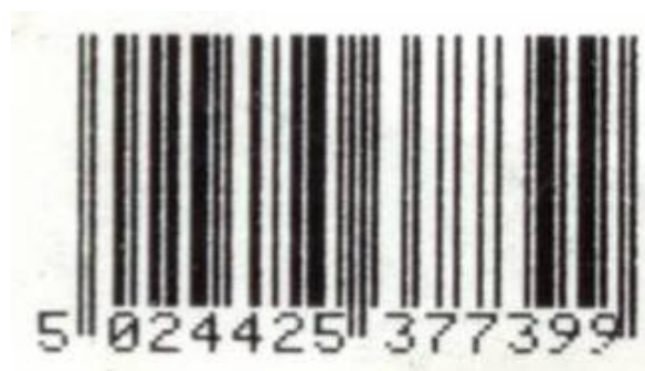
Figure 5.9.5.12-1. Symbol with edge determination problem
