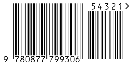
Figure 5.2.2.5.2-2. EAN-13 barcode with five-digit add-on symbol
