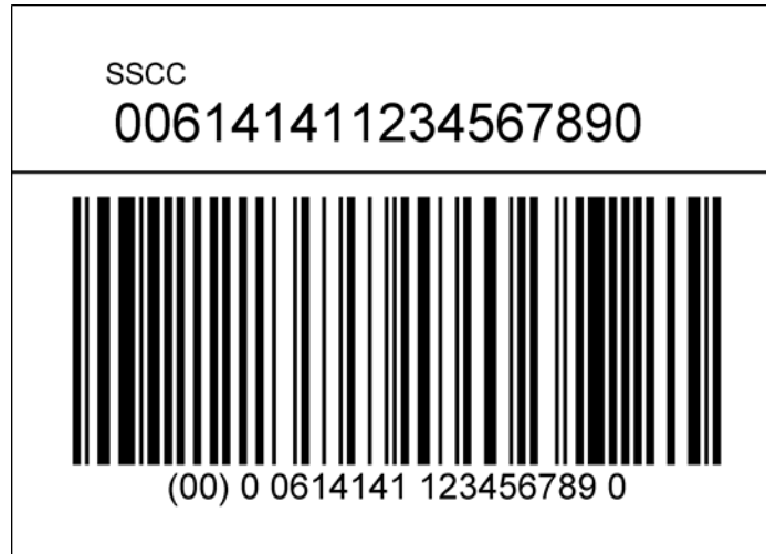
Figure 6.6.5-1. The basic label: an SSCC
