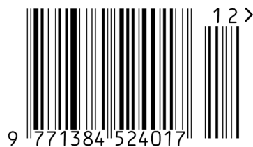
Figure 5.2.2.5.1-2. EAN-13 barcode with two-digit add-on symbol
