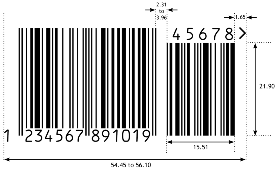
Figure 5.2.6.6-6. EAN-13 barcode with five-digit add-on symbol
