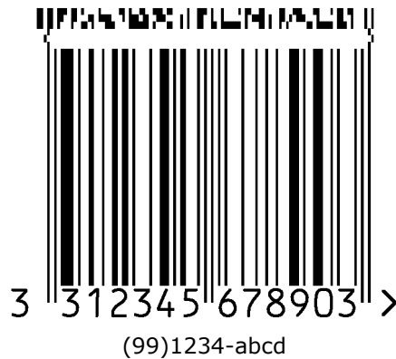
Figure 5.8.8-1. EAN-13 symbol with a four-column CC-A component
