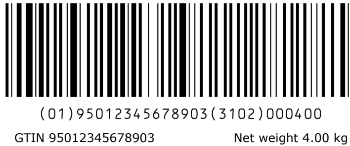
Figure 7.8.5.1-2. Data encoded in one concatenated GS1-128 symbol
