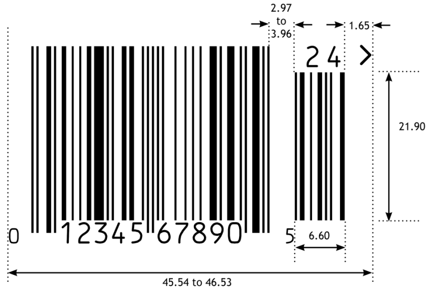
Figure 5.2.6.6-5. UPC-A barcode with two-digit add-on symbol
