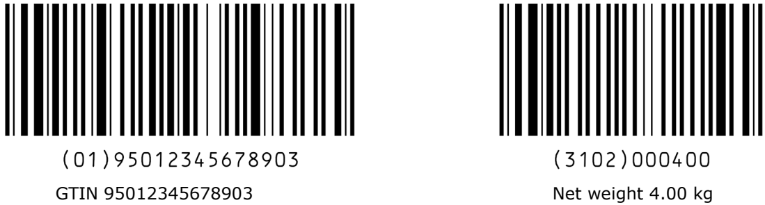
Figure 7.8.5.1-2. Data encoded in one concatenated GS1-128 symbol
