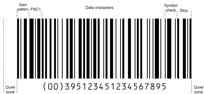
Figure 5.4.2-1. General format of a GS1-128 barcode
