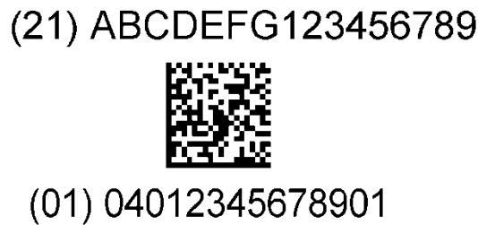
Figure 2.1.11-4. Example of GS1 DataMatrix symbol encoded with GTIN and serial number AI (21)
