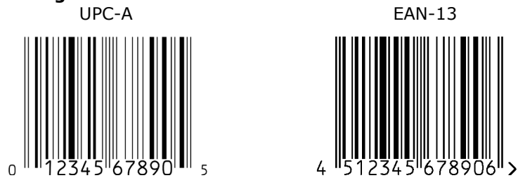
Figure 5.1-1. UPC-A and EAN-13 barcodes
