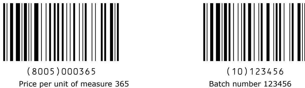
Figure 7.8.5.2-1. Data encoded in two GS1-128 symbols
