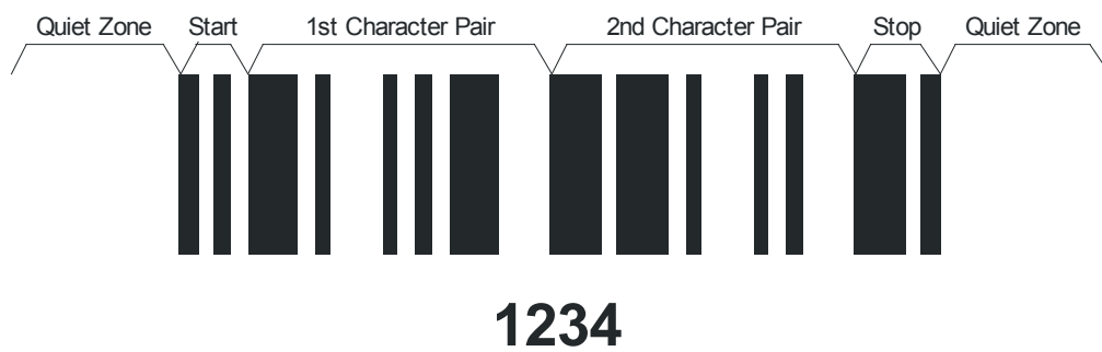
Figure 5.3.2.1.2-2. ITF-14 symbol inclusive of Quiet Zones
